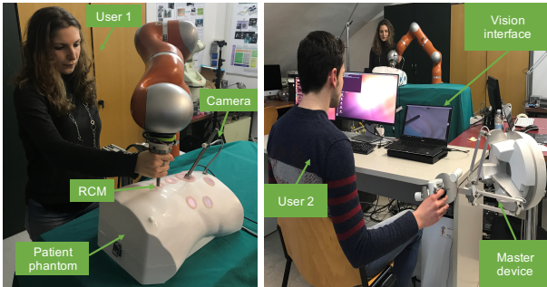
Fig. 3. Experimental setup procedures: Firstly, hands-on control is utilized to allow user 1 locate the RCM constraint by hand on the patient phantom; then user 2 use the master device to control the tool tip for surgical tasks.
